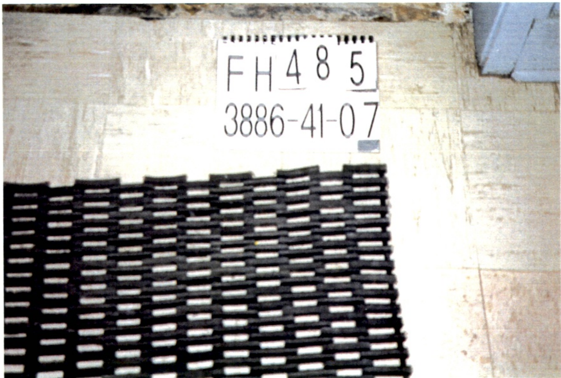
Bldg. 2525 Corridor 21A: Sample FH485, 12 x 12" tan floor tiles tested positive.
