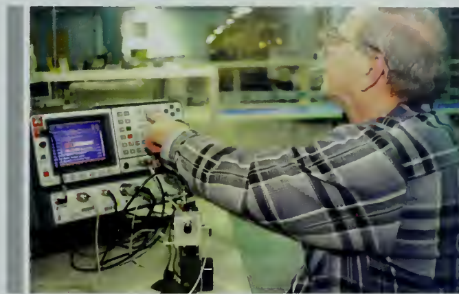
An electronics mechanic at Tobyhanna Army Depot tests the AN/PRC-112D pilot survival radio
